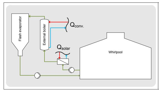
Example how to integrate solar heat for a wort boiling process in breweries.
